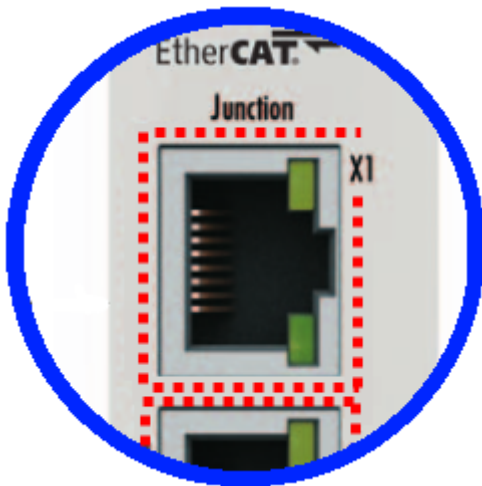
Fig. 10: Fast-Hot-Connect ports at the EK1122-0080
