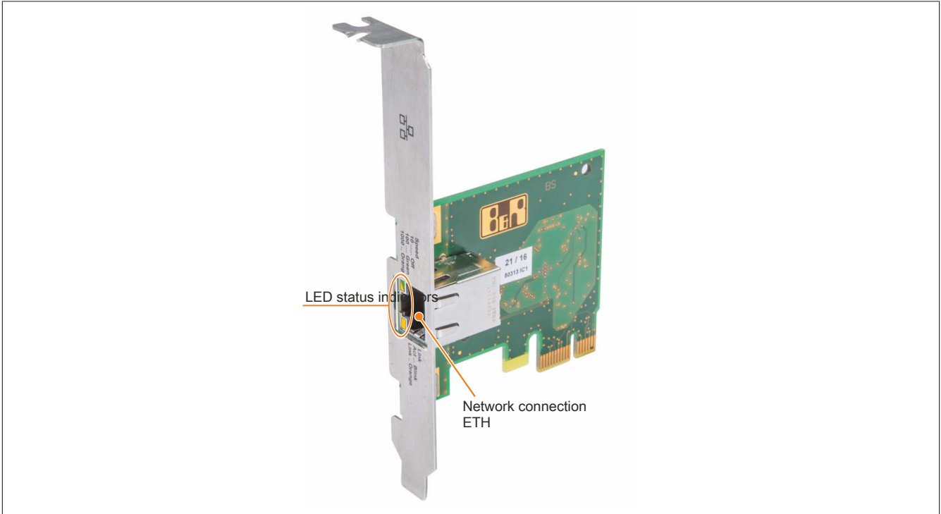
Figure 229: 5ACPCE.ETH1-00 - PCIe Ethernet card 10/100/1000
